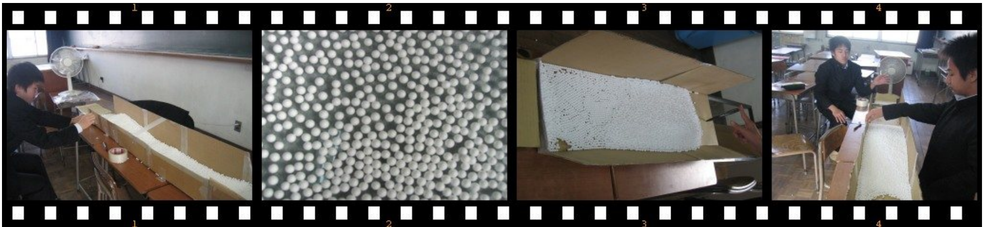
Fig14. A sand dune model using polyethylenes balls.
