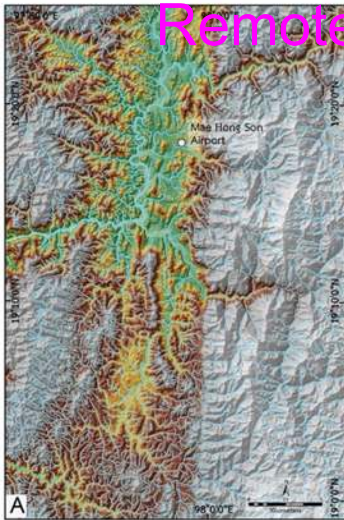
Figure 17 Detail interpreted map from ALOS DEM at Ban Pha Bong show offset stream of Sa Mad river is about 7.9 km, from right lateral strike-slip fault movement. Location shows in Figure 16B.
