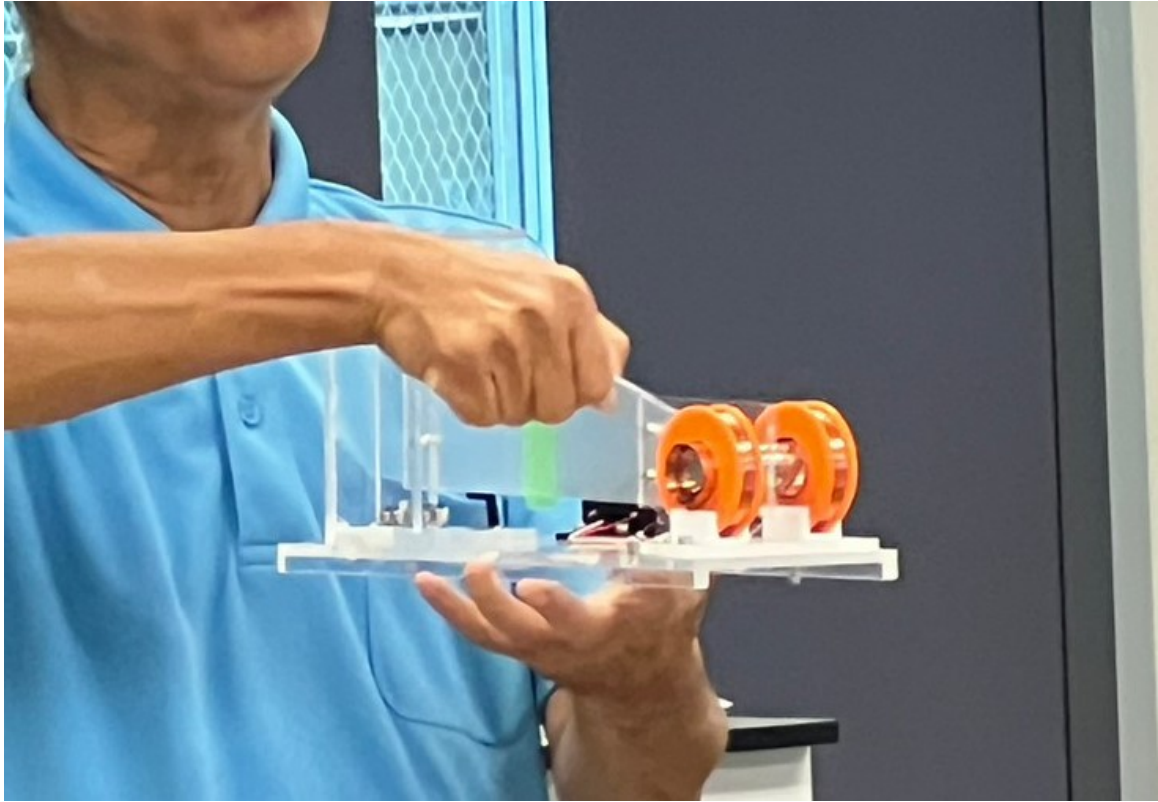
Figure 1: My hand-made “Skelton Seismometer” [4] to show the mechanism of seismograph.
