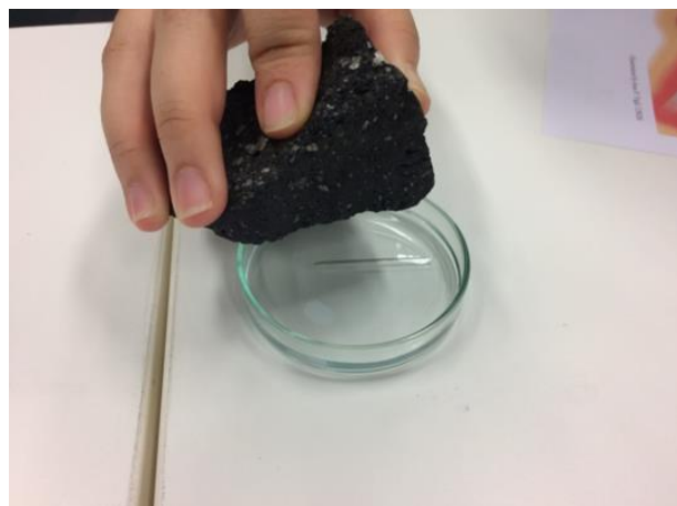
Figure.10 Thermal remnant magnetism of a basalt
