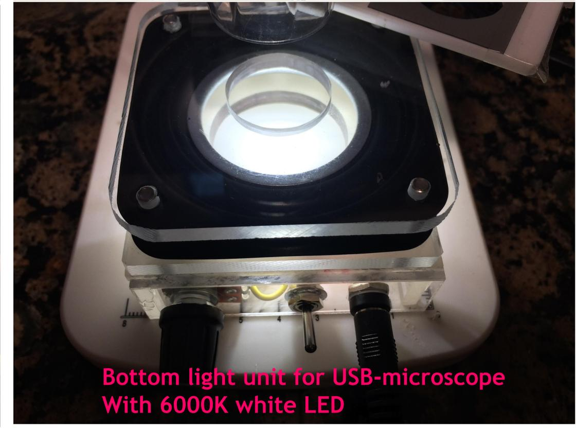
Bottom light unit for USB-microscope
