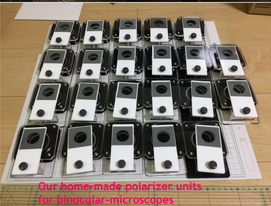
Our home-made polarizer units for binocular-microscopes
