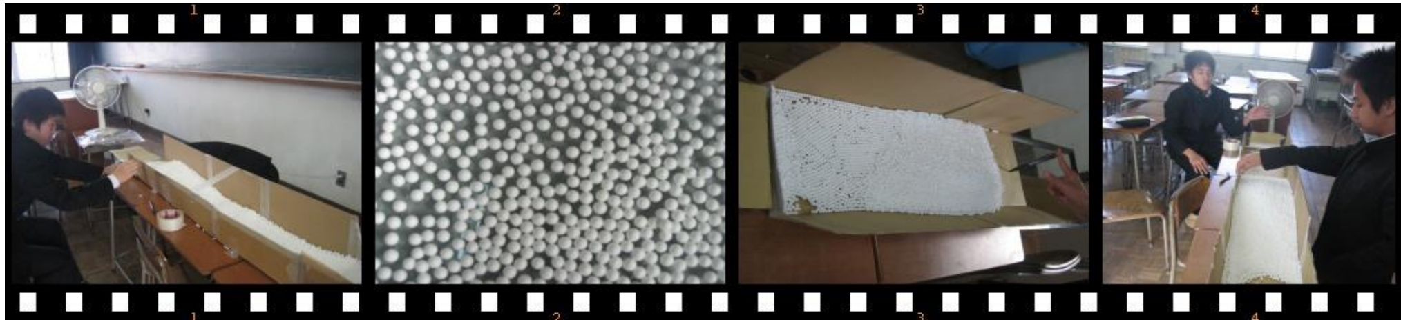
Fig14. A sand dune model using polyethylenes balls.
